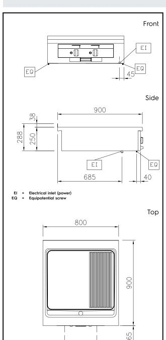
Electric Supply voltage: 400 V/3N ph/50/60 Hz Total Watts: 15.3 kW **Key Information:** Cooking Surface Depth: 615 mm Cooking Surface Width: 700 mm Working Temperature MIN: 80 °C 280 °C Working Temperature MAX: External dimensions, Width: 800 mm External dimensions, Depth: 900 mm External dimensions, Height: 250 mm Net weight: 120 kg One-Side Operated;Top Configuration: Cooking surface type: half ribbed/ half smooth Chromium Plated mild steel
